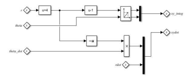
Once the angle of the pole vaulter, theta, becomes less than pi/2, the transition from Take\_off to Fly occurs. During the transition InitFly is initialized, the State Reader block connects to its owner block, and the function is executed. This function converts the polar coordinates from r, theta, and theta\_dot to Cartesian coordinates, xy\_integ and xydot. These coordinates are output as State Writer blocks, which are connected to owner blocks in the state Fly.
