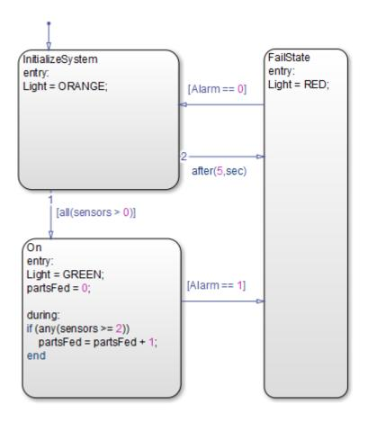
**Note** The outgoing transitions from InitializeSystem have a small label 1 and 2 to indicate the order in which transition segments are evaluated. If the numbers from the figure do not match your model, right click the transition and then change it by clicking on Execution Order. See "Transition Evaluation Order" on page 3-52 for details.
