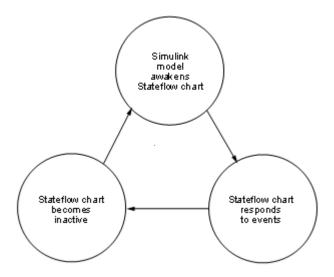
Because a chart runs on a single thread, actions that take place based on an event are atomic to that event. All activity caused by the event in the chart finishes before execution returns to the activity that was taking place before receiving the event. Once an event initiates an action, the action completes unless interrupted by an early return.
