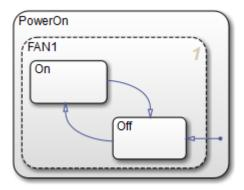
In this example, the tail of the default transition resides in PowerOn, not in FAN1. Therefore, it will activate FAN1 instead of FAN1.0ff.
