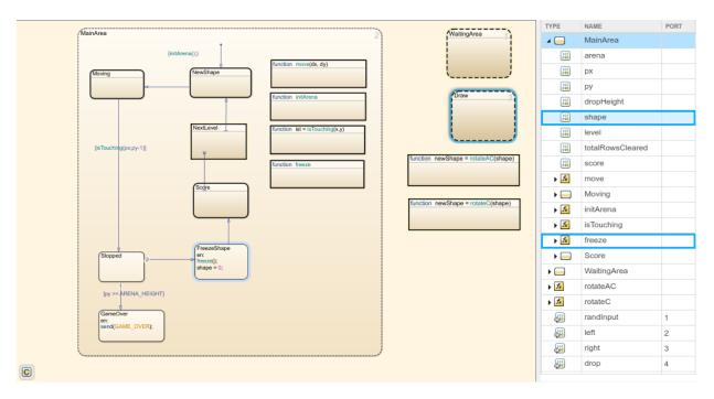
When in debugging mode, the values of each data are displayed in the **VALUE** column of the Symbols pane. Stateflow updates the values periodically when the simulation is running. The value column highlights changes to data values as the changes occur. When the debugger is stopped at a breakpoint, you can update the initial value or change the value of a symbols in either the command prompt or the Symbols pane.
