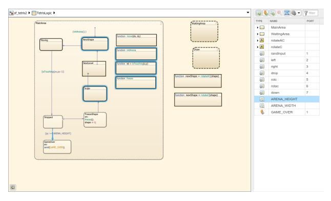
To see the uses of the constant ARENA\_HEIGHT, open the function freeze.
