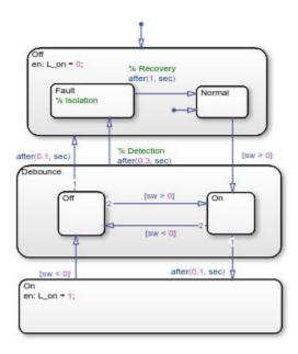
The debouncer design uses the after(n, sec) statement to implement absolute-time temporal logic. The keyword sec defines simulation time that has elapsed since activation of a state.
