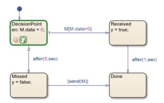
The initial value of the message is zero. To change the value of the data field to a positive number and send the message to its local queue, enter:
