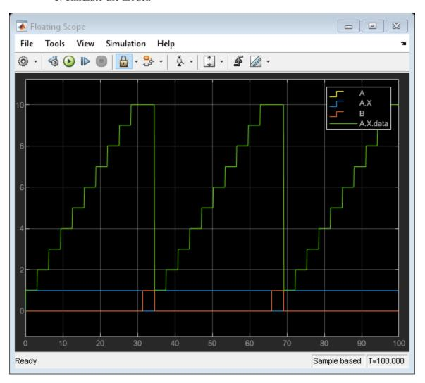
When state A.X is active, the signal value is 1. When that state is inactive, the signal value is 0. Because this value can be very low or high compared to other data, you might want to add a second Floating Scope block to compare the activity signal with other data.
