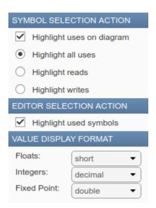
For Stateflow to highlight symbols in the Symbols pane that an object uses, select **Highlight used symbols.** For Stateflow to highlight objects in the chart that use an symbol, select **Highlight uses on diagram**. With **Highlight uses on diagram** you can choose to highlight:
