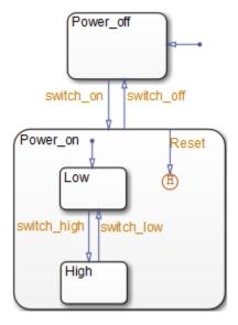
State Power\_on.High is initially active. When event Reset occurs, the inner transition to the history junction is valid. Because the inner transition is valid, the currently active state, Power on.High, is exited. When the inner transition to the history junction is
