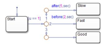
The chart uses temporal logic to determine when the input u equals 1.
