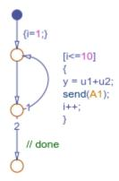
Each broadcast of the event A1 executes the subsystem A1. The subsystem computes its output and returns control back to the Loop Scheduler chart.
