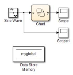
To access global data from a chart, bind a Stateflow data object to a Simulink data store. After you create the binding, the Stateflow data object becomes a symbolic representation of the Simulink data store memory. You can then use this symbolic object to store and retrieve global data.
