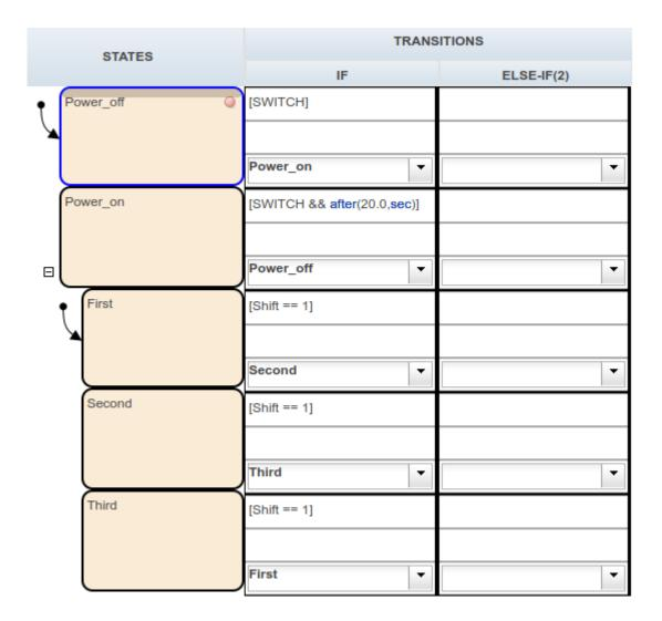
Now the transition from Power\_on to Power\_off does not occur until 20 seconds have passed.
