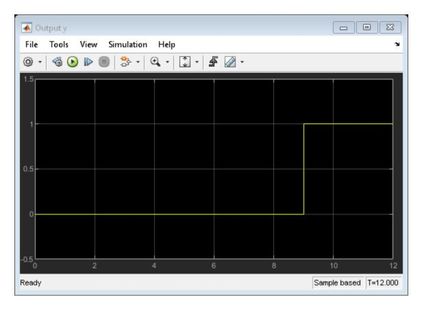
This model behavior applies only to subsystems where you set the Enable block parameter **States when enabling** to held. If you set the parameter to reset, the chart reinitializes completely when the subsystem is reenabled. In other words, default transitions execute and any temporal logic counters reset to 0.
