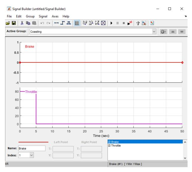
However, this approach has limitations. The signal changes value based on time, but cannot respond dynamically to changes in the system that are not governed by time alone. For example, how does the signal know when the transmission shifts into the highest gear? In this case, the signal assumes that the shift always occurs at time 5
