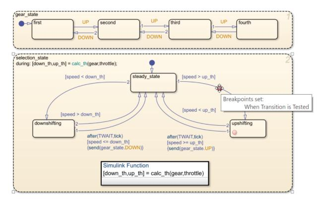
To inspect the chart before the transition is taken, you want the breakpoint to pause the simulation only when the value of speed is approaching the value of up\_th. When you set the condition speed > up\_th-2 on the breakpoint, the simulation pauses only when the value of speed is within 2 of the value of up\_th.
