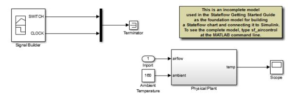
The model is incomplete because it does not include the Stateflow chart that you will build as you work through the exercises in this guide. Instead, the model contains several nonfunctional blocks: the Terminator, Inport, and Annotation blocks.
