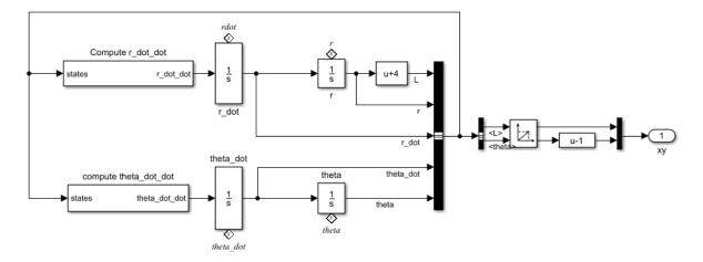
Once the position of the pole vaulter along the x-axis, Run\_up.p(1), becomes greater than -4, the active state becomes Take\_off. This Simulink subsystem models the pole vaulter during the take off phase of the jump. The subsystem outputs the Cartesian coordinates of the pole vaulter.
