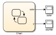
The outputs of a sampled Stateflow block are held after the execution of the block.
