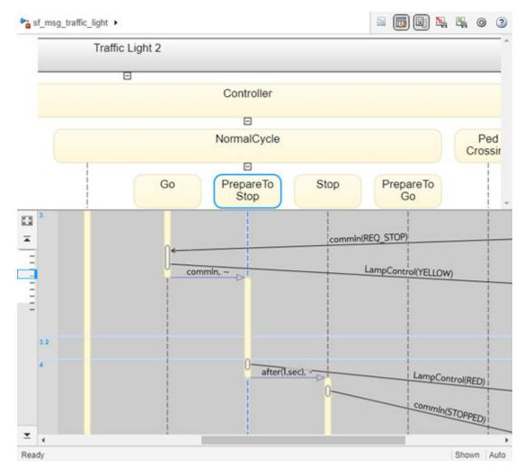
To display the start state, end state, and full transition label in the Property Inspector, click the arrow corresponding to the transition.
