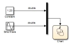
You cannot mux two input signals of different data types, such as boolean and double.
