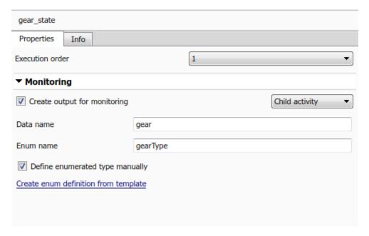
The enumeration data type definition contains one literal for each state name plus an extra literal to indicate that no substate is active. For example, in the model sf\_car, the state gear\_state contains four child states that correspond to the gears in a car: first, second, third, fourth. The model specifies the child activity data type with this enumeration class definition:
