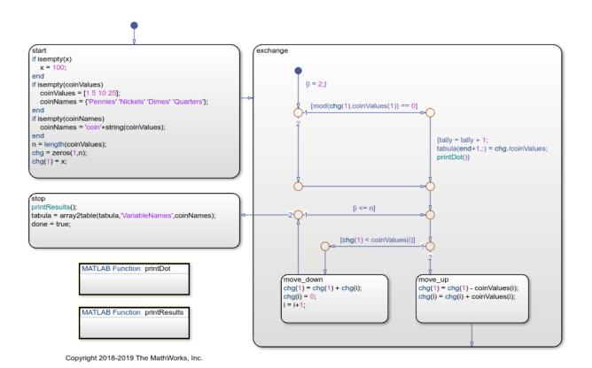
The chart begins with a potential change configuration consisting entirely of the lowest-value coins, specified by an index of 1. At each execution step, the state exchange modifies this configuration in one of two ways:
