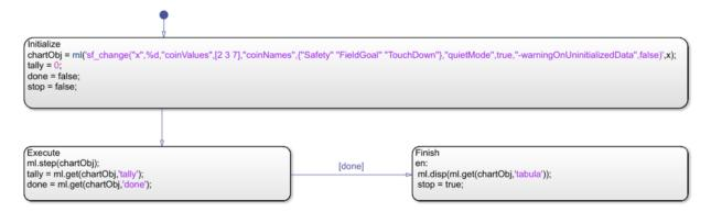
When you simulate this chart with an input of x = 27, the Display block Modern American shows a tally of 13. The Diagnostic Viewer window shows these results:
