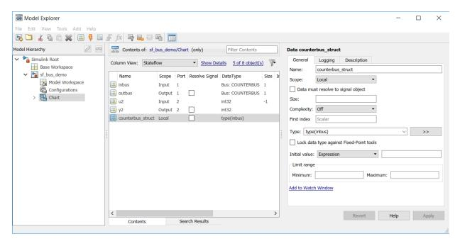
After you build your model, the **CompiledType** column of the Model Explorer shows the type used in the compiled simulation application.
