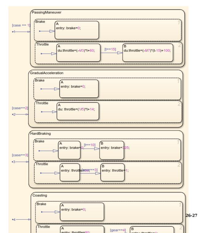
In some of these scenarios, the throttle changes in response to time; in other cases, it responds to gear selection, an output of the Stateflow chart Shift logic. The Shift logic chart determines the gear value based on the speed of the vehicle.
