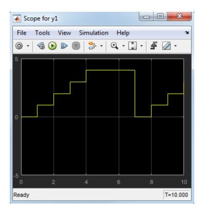
When state A1 becomes inactive at t=5, the Simulink function does *not* hold the counter value. When A1 is active again at t=7, the counter resets to zero. Therefore, the output y1 resets too.
