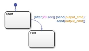
When simulation starts, the value of the trigger signal is 0. At time t=20, the chart dispatches output\_cmd, changing the value of the trigger signal to 1. The enabled subsystem becomes active and executes during that time step. The chart queues up the second event for dispatch at the next time step. At time t=21, the chart dispatches the
