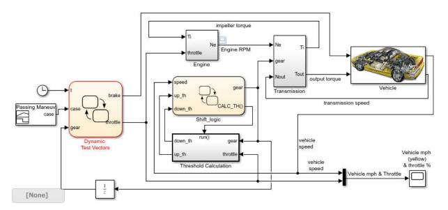
The chart models the dynamic relationship between the brake and throttle to test four driving scenarios. Each scenario is represented by a state.
