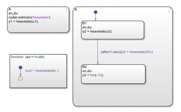
You only need to declare heaviside once in your chart using coder.extrinsic. After this you can use the heaviside function anywhere within your chart without coder.extrinsic. When generating code the functions that you declare using coder.extrinsic will have a call to the extrinsic function, and that function will not appear in the generated code.
