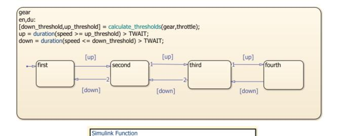
[down\_th,up\_th] = calculate\_thresholds(gear,throttle)
