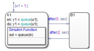
The function queue contains a block diagram that increments a counter by 1 each time the function executes.
