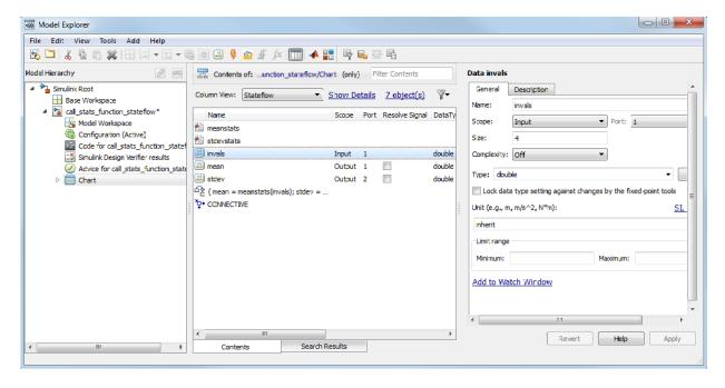
After you add the data invals, mean, and stdev to the chart, the corresponding input and output ports appear on the Stateflow block in the model.
