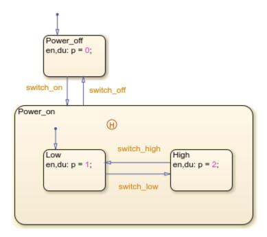
By following the "Workflow for Entering a Chart or State" on page 3-37 until the chart goes to sleep, the execution steps for entering the state Power on are in this order:
