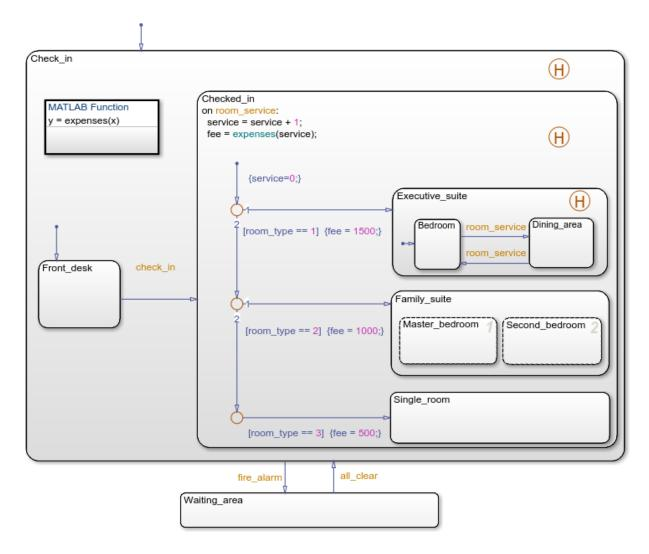
A transition from the Front\_desk state to a connective junction is labeled by the check\_in event. Transitions from the connective junction to the destination states are labeled with conditions. If Front\_desk is active when check\_in occurs, the transition from Front\_desk to the connective junction occurs first. The transition from the
