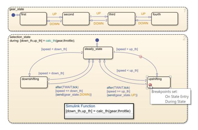
To change the type of breakpoint on an object, click the breakpoint badge. In the Breakpoints dialog box, you can select a different configuration of breakpoints, depending on the object type.
