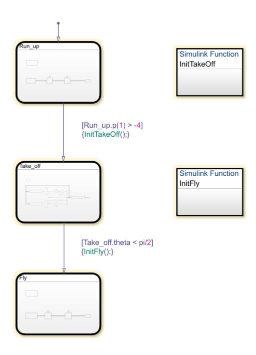
The states Run\_up and Fly are easier to model by using Cartesian coordinates. The state Take\_off is easier to model by using polar coordinates. To switch from one coordinate system to another, use Simulink functions InitTakeOff and InitFly.
