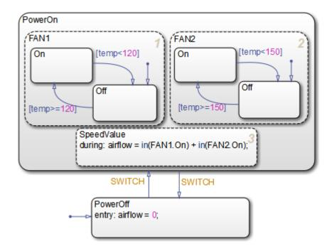
Now that you have associated these transitions with the event SWITCH, the control system will alternately power on and off every time SWITCH occurs — that is, every time the chart detects a rising or falling signal edge.
