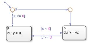
The default transition to the connective junction defines that upon entering the chart, the destination depends on the condition of each transition segment.
