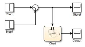
In this model, the Sum block produces a 2-by-1 vector signal that goes from [0,0] to [1,1] at time t=1. As a result, when the model wakes up the chart, events E1 and E2 are both active:
