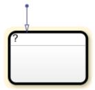
4 Enter the state label. In this example, the state models a pole vaulter running along a flat surface, so the state label is Run\_up. Simulink based states are action subsystems, so an Action Port appears with your new state.
