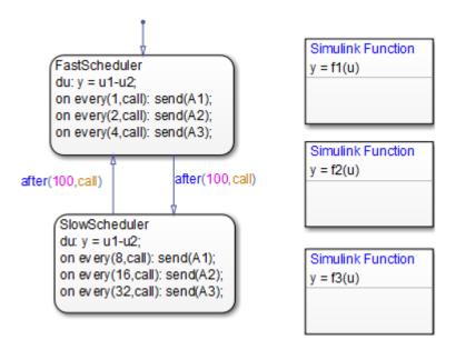
**Note** The new functions reside at the chart level because both states FastScheduler and SlowScheduler require access to the function outputs.
