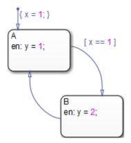
In this example, the transitions between states A and B cycle and produce an infinite loop because the value of x remains constant at 1. One way to detect infinite loops is to configure your chart to generate an error if it reaches a maximum number of iterations in a super step. See "Enable Super Step Semantics" on page 3-60.
