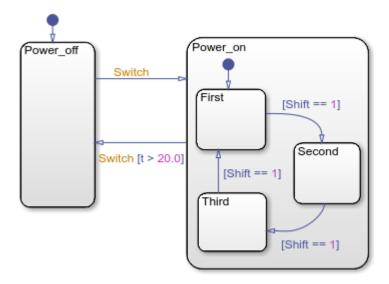
Now the transition from Power\_on to Power\_off does not occur until simulation time is greater than 20.0.
