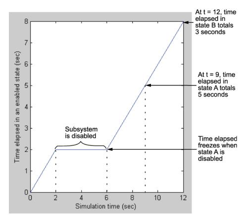
When the input signal enables the subsystem at time t = 0, the state A becomes active, or enabled. While the state is active, the time elapsed increases. However, when the subsystem is disabled at t = 2, the chart goes to sleep and state A becomes inactive.
