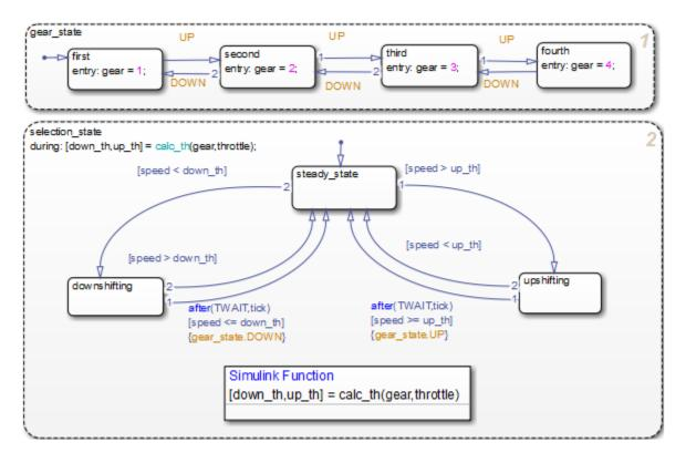
In the chart, the during action in selection\_state contains a function call to calc th, which is a function that contains Simulink blocks.
