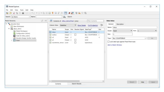
The main window has two panes: a **Model Hierarchy** pane on the left and a **Contents** pane on the right. When you open the Model Explorer, the Stateflow object you are editing appears highlighted in the **Model Hierarchy** pane and its objects appear in the **Contents** pane. This example shows how the Model Explorer appears when opened from the chart.
