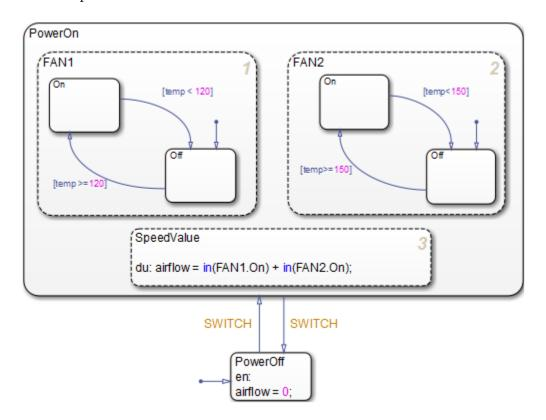
Without the default transition to state PowerOff, when the Stateflow chart wakes up, none of the states becomes active. A state inconsistency error is reported at run time.
