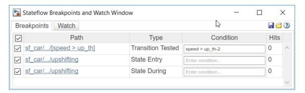
When the simulation pauses, you can inspect the values of the variables speed and up\_th and step through the simulation. For more information, see "Inspect and Modify Data and Messages While Debugging" on page 32-12 and "Control Chart Execution After a Breakpoint" on page 32-21.
