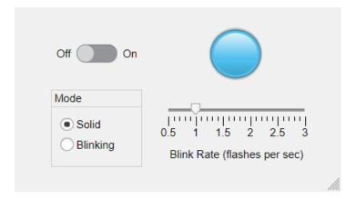
The file sf\_lamp\_logic.sfx defines a standalone Stateflow chart that implements the logic for the user interface. The chart has input events (ON, OFF, BLINKING, and SOLID) and local data (delay and app). The actions in the chart control which widgets are accessible from each state. For instance, the actions in the Off state cause the Lamp widget, the Mode option buttons, and the Blink Rate slider in the user interface to appear dimmed.
