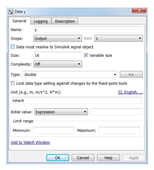
As in the chart VarSizeSignalSource, variable-size data does not appear in state actions or transition logic. Instead, states call MATLAB functions to compute the variable-size output. Transitions call a MATLAB function in a conditional statement to evaluate the variable-size input.
