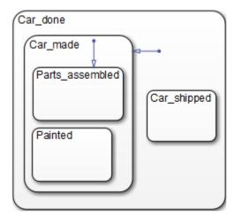
In this example, the chart is the parent of the state Car\_done. The state Car\_done is the parent state of the Car\_made and Car\_shipped states. The state Car\_made is also the parent of the Parts\_assembled and Painted states. You can also say that the states Parts\_assembled and Painted are children of the Car\_made state.
