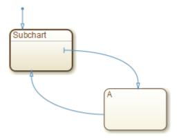
**Note** If the parent chart is itself a subchart and the terminating object resides at a higher level in the subchart hierarchy, repeat these steps until you reach the desired parent. In this way, you can connect objects separated by any number of layers in the subchart hierarchy.
