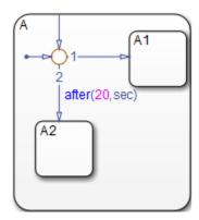
In this example, state A has both an inner and a default transition that connect to a junction with outgoing transitions to states A.A1 and A.A2. If state A is active, its set of inner flow charts includes:
