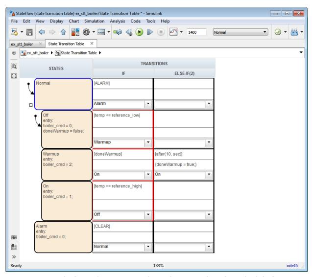
3 To view the flow in the autogenerated state diagram, in the Debug tab, click Show Auto Chart.
