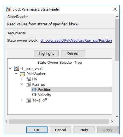
**3** By connecting the State Reader block to the Position integrator block, this Simulink function can use the state of the integrator Position to execute.
