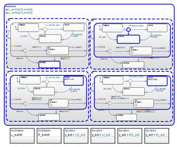
This mode logic assumes that there are 3 hydraulic lines, one that is connected to the 2 redundant actuators (Left Inner and Right Inner actuators).
