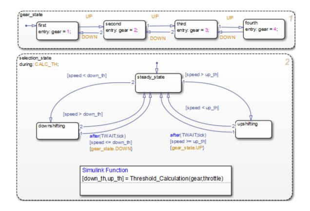
**Note** The function resides in this state instead of the chart level because no other state in the chart requires the function outputs up\_th and down\_th. See "Bind a Simulink Function to a State" on page 29-19.
