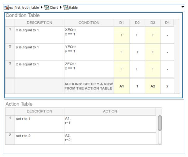
• Row number action specifiers in the **Actions** row of the **Condition Table** automatically adjust to changes in the row order of the **Action Table**.
