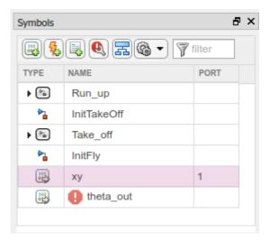
5 Stateflow creates an output in the chart called theta\_out that corresponds to the outport theta\_out.
