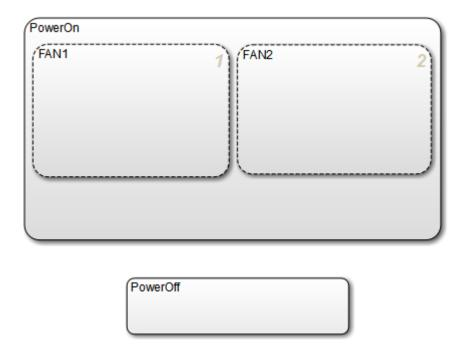
**Note** Your chart might not show the same execution order for parallel substates FAN1 and FAN2. The reason is that, by default, Stateflow software orders parallel states based on order of creation. If you add FAN2 before FAN1 in your chart, FAN2 moves to the top of the order. You will fine-tune order of activation in a later exercise, "Setting Explicit Ordering of Parallel States" on page 1-39.
