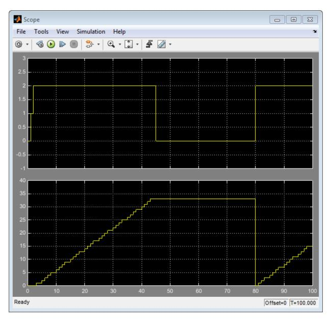
The upper axis shows the LED signal which varies between red (0), orange (1), and green (2) to indicate the current operating mode. The lower axis shows the number of parts fed
