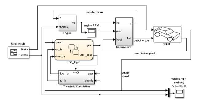
This model simulates for 30 seconds, but you want to see what happens when the value of gear changes at t = 10. You can simulate the model, save the operating point at t = 10, load and modify the operating point, and then simulate again between t = 10 and 20.
