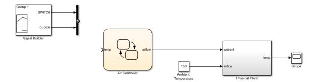
**Tip** You can use a shortcut for automatically connecting blocks. Select the source block, and then hold down the **Ctrl** key and left-click the destination block.
