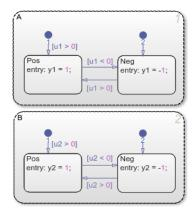
To enable reuse of subcomponents by using linked atomic subcharts, create a single copy of state A and store it as a chart in a library model. From that library, copy and paste the atomic subchart twice in your chart. Then update the mapping of subchart variables as needed.
