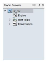
Click the double arrows in the bottom left corner to open or close a tree-structured view of the model in the editor.
