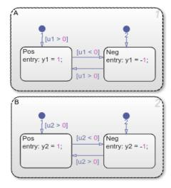
Suppose that you want to reduce the compilation time of the chart for simulation. You can convert state A to an atomic subchart. Then you can make changes, one by one, to state A
