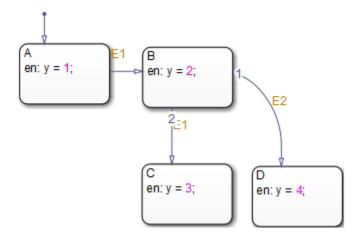
If you enable super step semantics, the chart takes all valid transitions for event E1. The chart takes transitions from state A to B and then from state B to C in a single super step. The scope shows that y = 3 at the end of the super step:
