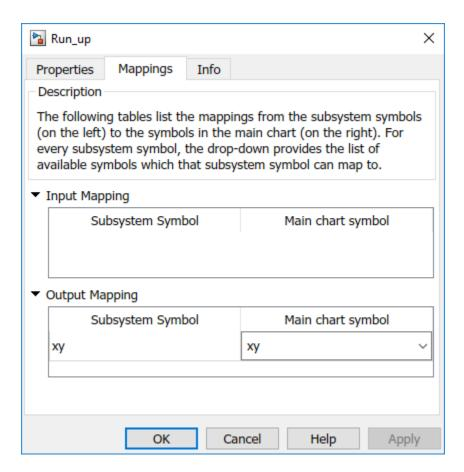
Under **Input Mapping**, you can specify which parent chart input maps to an inport in your Simulink subsystem.
