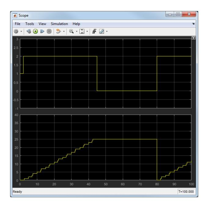
The upper axis shows the LED signal which varies between orange (1), green (2), and red (0) to indicate the current operating mode. The lower axis shows the number of parts fed to the next assembly station, which increases incrementally until the alarm signal turns the machine off and then resets.
