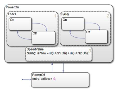
**5** Repeat the same procedure to add default transitions at the top edges of FAN1.0ff and FAN2.0ff.
