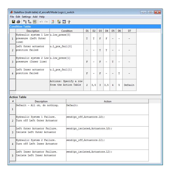
The first requirement indicates that if a failure is only detected in the hydraulic pressure 1 system, turn off the left outer actuator. This requirement is represented in the decision D1 in the truth table. If there is low pressure in the hydraulic system 1, then D1 specifies that action 2 is performed. Action 2 sends an event go\_off to the left actuator, Actuators.L0.
