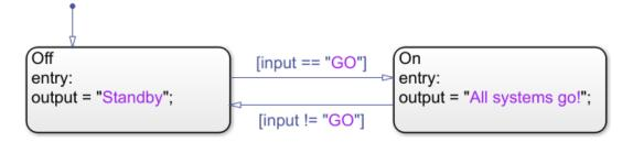
To specify a string symbol, set its **Type** field to string. Stateflow dynamically allocates memory space for this type of data.
