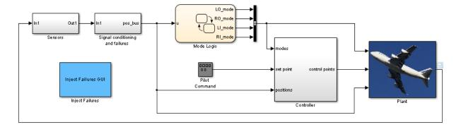
The Mode Logic chart monitors the status of actuators for two elevators. Each elevator has an outer (primary) actuator and an inner (secondary) actuator. In normal operation, the outer actuators are active and the inner actuators are on standby.
