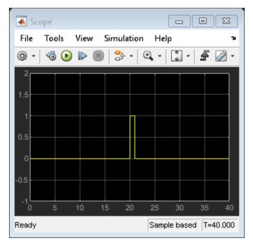
Although you can approximate a function call, there is a subtle difference in execution behavior. Execution of a function-call subsystem occurs *during* execution of the chart action that provides the trigger. Execution of an enabled subsystem occurs *after* execution of the chart action is complete.
