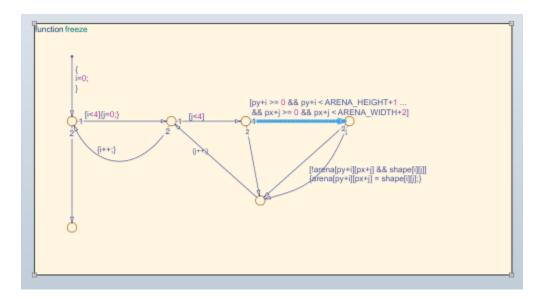
You can also select a graphical object such as a state, transition, or function in the chart and view the symbols that the object uses. For example, in the chart TetrisLogic, expand the symbol MainArea in the Symbols pane. If you select the state FreezeShape in the chart, then the local data shape and the function freeze() are highlighted in the Symbols pane. This highlighting indicates that those objects are used inside the state FreezeShape.
