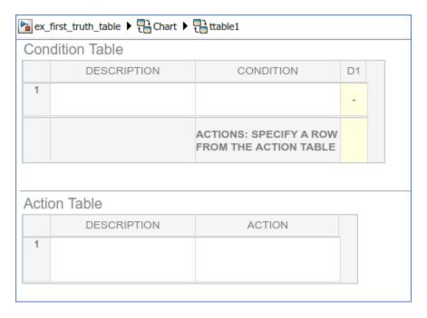
By default, a truth table contains a **Condition Table** and an **Action Table**, each with one row. The **Condition Table** contains a single decision column, **D1**, and a single action row.
