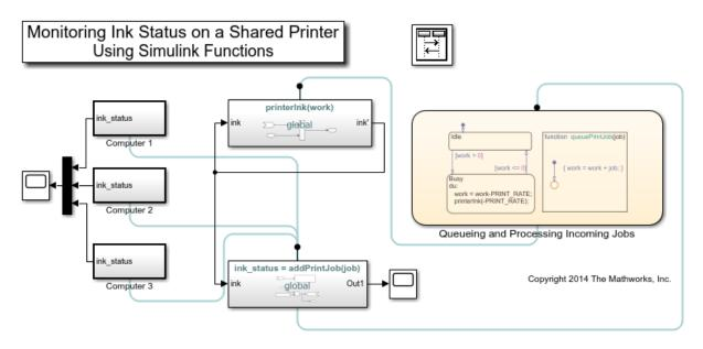
Each computer client invokes the printer server with a call to the Simulink function, addPrintJob. The addPrintJob function calls the Stateflow graphical function queuePrintJob to add the print job to the work load. The chart processes the work and calls the Simulink function printerInk to model usage of printer ink.
