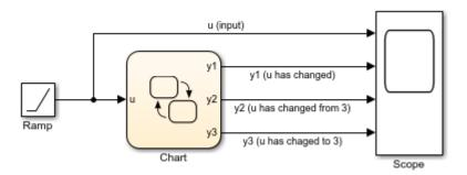
The model uses a fixed-step solver with a step size of 1. The signal increments by 1 at each time step. At each time step, the chart analyzes the input signal u for these changes:
