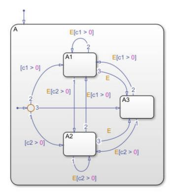
Any event occurs and awakens the Stateflow chart. The default transition to the connective junction is valid. The destination of the transition is determined by [c1 > 0] and [c2 > 0]. If [c1 > 0] is true, the transition to A1 is true. If [c2 > 0] is true, the transition to A2 is valid. If neither [c1 > 0] nor [c2 > 0] is true, the transition to A3 is valid. The transitions among A1, A2, and A3 are determined by E, [c1 > 0], and [c2 > 0].
