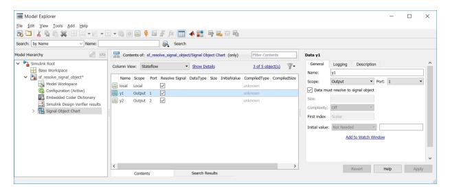
When you build the model, each data object inherits the properties of the identically named signal.
