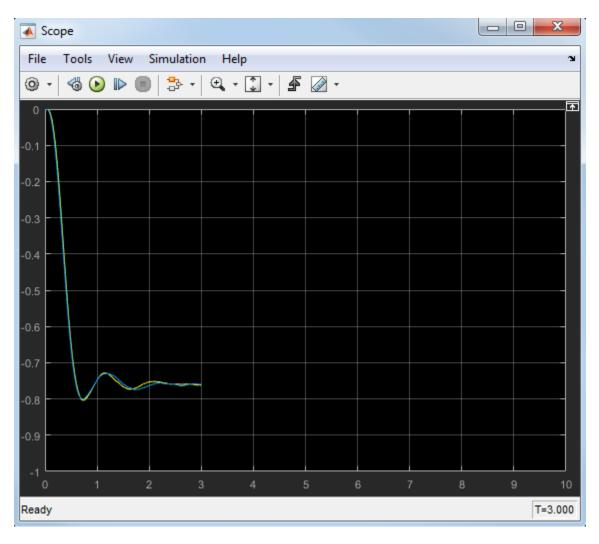
Suppose that you want to see what happens at t=3 when at least one actuator fails. You can simulate the model, save the operating point at t=3, load and modify the operating point, and then simulate again between t=3 and 10.
