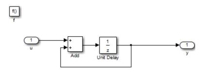
At each time step, the function f is called twice, which causes the counter to increment by 2. Because all call sites share the value of this counter, the data y and y1 increment by 2 at each time step.
