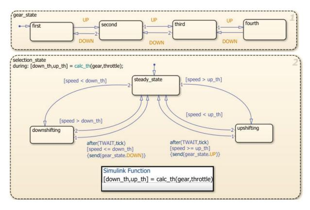
In this Stateflow chart, for the car to move from first gear to second gear, the event UP must be sent from selection\_state to gear\_state. The event is sent when the speed crosses the threshold and remains higher than the threshold for the length of time determined by TWAIT. When the event UP is sent, gear\_state transitions from first to second.
