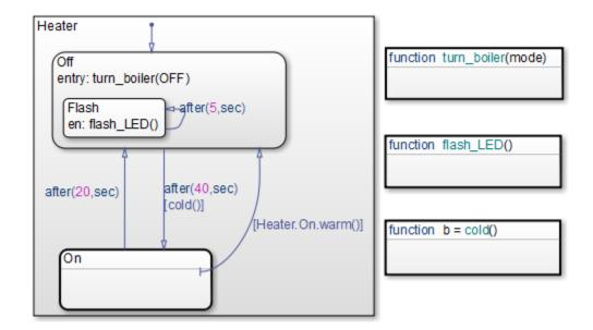
If the parser cannot resolve a syntax element, the chart displays the element in the default text color.
