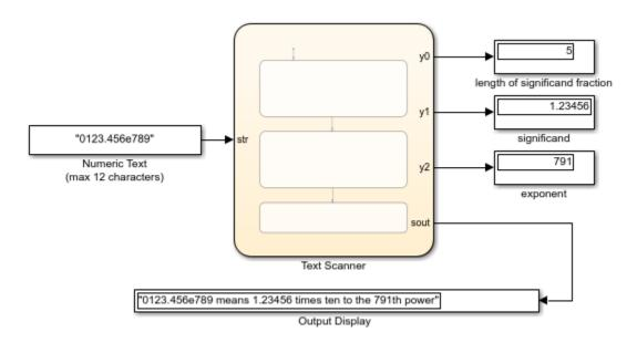
This model contains a Stateflow chart that calls two functions from custom C code. During simulation, the chart takes as its input a string that contains text representing a floating-point number in exponential form. The chart consists of three states that:
