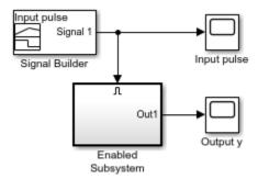
The subsystem contains a chart that uses the after operator.
