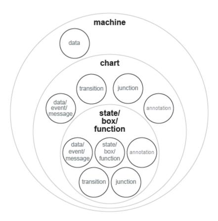
The highest object in Stateflow hierarchy is the Stateflow machine. The Stateflow machine contains all of the Stateflow charts in a Simulink model. In addition, the Stateflow machine for a model can contain its own data.
