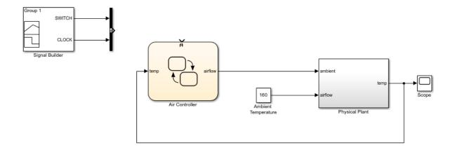
When you define one or more input events for a chart, Stateflow software adds a single trigger port to the block. External Simulink blocks can trigger the input events via a signal or vector of signals connected to the trigger port.
