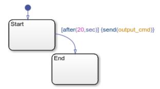
When simulation starts, the value of the trigger signal is 0. At time t=20, the chart dispatches output\_cmd, changing the value of the trigger signal to 1. The enabled subsystem becomes active and executes during that time step. Because no other event broadcasts occur, the enabled subsystem continues to execute at every time step until simulation ends at t=40. The Display block shows a final value of 40.
