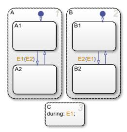
Because undirected local event broadcasts can cause unwanted recursive behavior, use of the send operator to broadcast directed local events is recommended. For more information, see "Broadcast Local Events to Synchronize Parallel States" on page 12-46.
