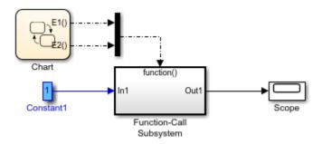
In the chart, E1 binds to state A, but E2 does not. State B sends the triggering event E2 in its entry action.
