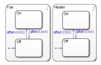
Fan and Heater are parallel (AND) superstates. The first time that an event awakens the Stateflow chart, the states Fan.Off and Heater.Off become active.
