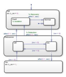
For details on how this chart works, see "Debounce Signals with Fault Detection" on page 26-7. For information on the semantics of this notation, see "Transition from a Substate to a Substate with Events" on page B-8.
