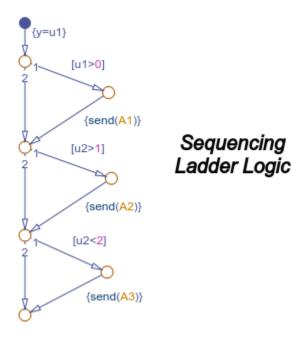
The chart evaluates each condition sequentially. When a condition is valid, the chart calls the send operator to broadcast an output event. The corresponding subsystem computes its output and returns control back to the Ladder Logic Scheduler chart.
