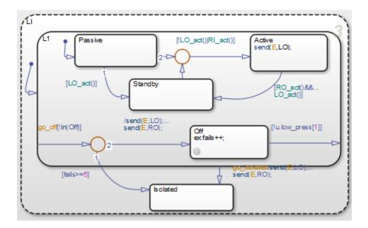
For the inner left actuator (LI ), the transition to Active inside the L1 superstate is conditionally based on [!L0\_act()|RI\_act()]. This causes the left inner actuator to turn on if the outer actuator (L0) has failed, or the right inner actuator (RI) has turned on.
