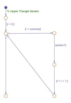
To complete the upper triangle iterator pattern, insert a second for loop along the vertical transition in this flow chart.
