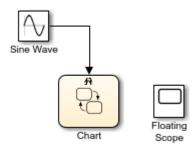
In the Stateflow chart, state A and its substate X are entered on the first tic event. State A and substate X stay active until 10 tic events have occurred, and then state B is entered. On the next event, state A and substate X are entered and the cycle continues. The data data belongs to substate X. The entry and during actions for substate X increment data while X is active for 10 tic events. When state B is entered, data reinitializes to zero, and then the cycle repeats.
