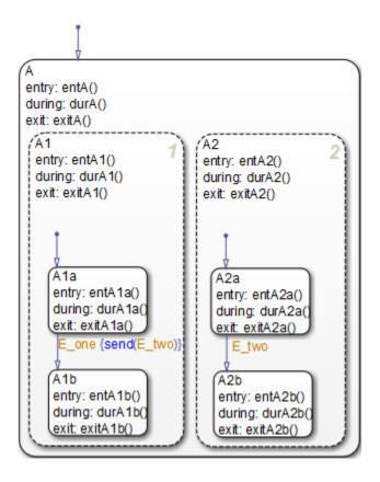
Initially, the chart is asleep. Parallel substates A.A1.A1a and A.A2.A2a are active. Event E\_one occurs and awakens the chart, which processes the event from the root down through the hierarchy:
