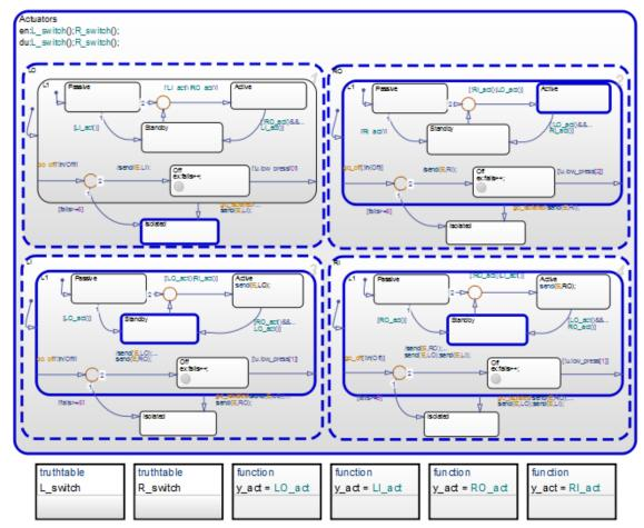
This mode logic assumes that these are 3 hydraulic lines, one that is connected to the 2 redundant actuators (Left inner and Right Inner actuators). The other two are connected to the primary actuators Left Outer and Right Outer (1 per actuator).
