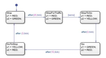
In the Moore chart, each state represents the colors of the traffic light in two opposite directions and the duration of the current color. Each state action computes output (the colors of the traffic light) regardless of input (if there are cars waiting at a sensor). If you change the chart type to Mealy, you get a compile-time diagnostic message indicating that the chart violates Mealy chart semantics. According to Mealy semantics, the chart cannot compute its outputs in state actions.
