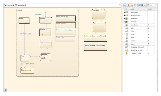
The rows in the Symbols pane display object hierarchy. Expand an object in the window to see data, events, and messages parented by that object. By default, all the nongraphical objects in a chart are listed in the window. To view only the objects that are used at the
