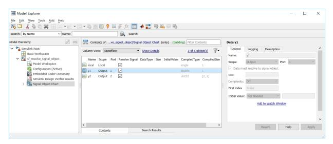
The generated code declares the data based on the storage class that the data inherits from the associated Simulink signal. For example, the header file below declares local to be an exported global variable:
