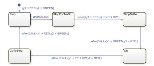
In the same time step, the Mealy chart evaluates the temporal logic expressions and the input signal sens, and computes the value of the outputs y1 and y2. As a result, in the Mealy chart, the output changes one time step before the corresponding change occurs in the original Moore chart. In the Simulink model, you can compensate for the anticipated changes in output by adding a Delay block to each output signal.
