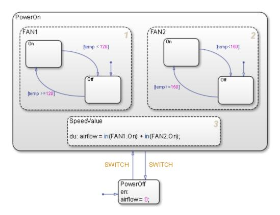
As you can see from the title bar, the chart is called Air Controller and is part of a Simulink model called sf\_aircontrol. When you build this chart, you will learn how to work with the following elements of state-transition charts:
