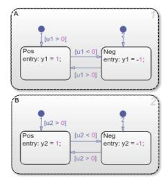
Suppose that you want to generate reusable code so that you can perform unit testing on state A. You can convert that part of the chart to an atomic subchart and then specify a separate file to store the generated code.
