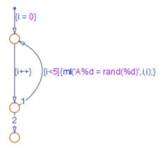
The for loop creates four new matrix variables in the MATLAB workspace. The default transition initializes the Stateflow counter i to 0, while the transition segment between the top two junctions increments it by 1. If i is less than 5, the transition segment back to the top junction evaluates the ml function call ml('A%d = rand(%d)',i,i) for the current value of i. When i is greater than or equal to 5, the transition segment between the bottom two junctions occurs and execution stops.
