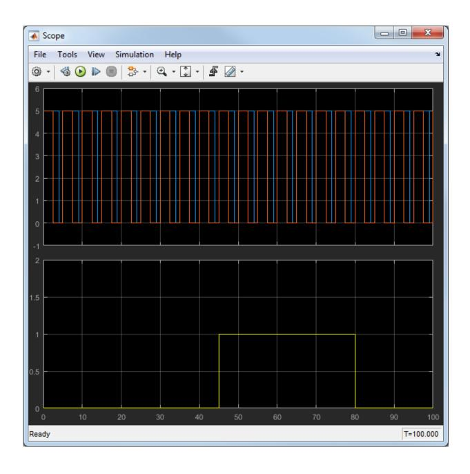
The upper axis shows the sensor signals. Only two sensor signals appear because two of the sensors have the same signal. The lower axis shows the alarm signal which turns the feeder off between the simulation time of 45 to 80 seconds.
