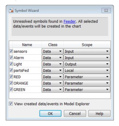
The Symbol Wizard does not automatically add any data to your chart. It identifies the unresolved data and infers the class and scope of that data using the inference rules of MATLAB expressions in Stateflow actions. In the chart:
