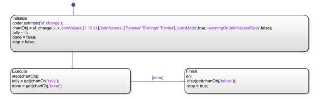
When you simulate this chart with an input of x = 27, the Display block Olde English shows a tally of 4. The Diagnostic Viewer window shows these results:
