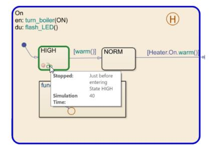
To view the values of chart, point to a chart object. A tooltip displays:
