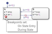
To change the type of breakpoint on an object, click the breakpoint badge. In the Breakpoints dialog box, you can select a different configuration of breakpoints, depending on the object type. Clearing all of the check boxes in the Breakpoints dialog box removes the breakpoint.
