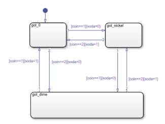
In the Mealy chart, each state represents one of the three possible coin inputs: nickel, dime, or no coin. Each condition action computes output (whether soda is released) based on input (the coin received) as the chart transitions to the next state. If you change the chart type to Moore, you get a compile-time diagnostic message indicating that the chart violates Moore chart semantics. According to Moore semantics, the chart output soda cannot depend on the value of the input coin.
