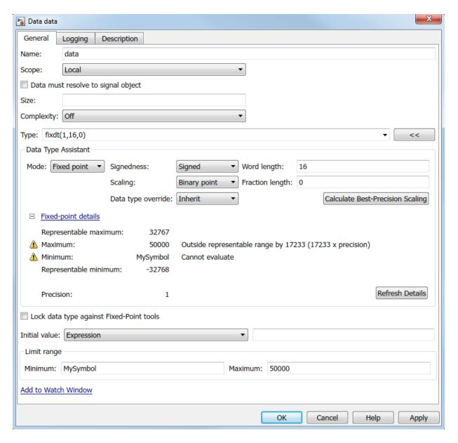
The row labeled Maximum indicates that the value specified in the **Maximum** field of the **Limit range** section is not representable by the fixed-point data type. To correct the
