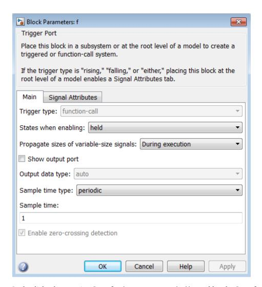
In the dialog box, setting **Sample time type** to periodic enables the **Sample time** field, which defaults to 1. These settings tell the function to execute for each time step specified in the **Sample time** field while the function is enabled.
