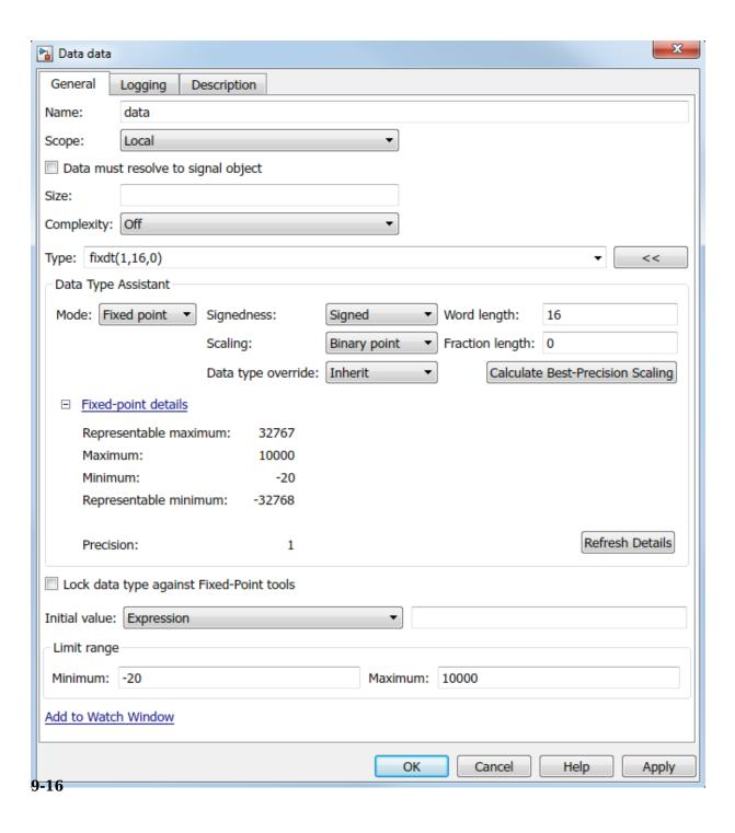
The values displayed by the **Fixed-point details** subpane *do not* automatically update if you change the values that define the fixed-point data type. To update the values shown in the **Fixed-point details** subpane, click **Refresh Details**.
