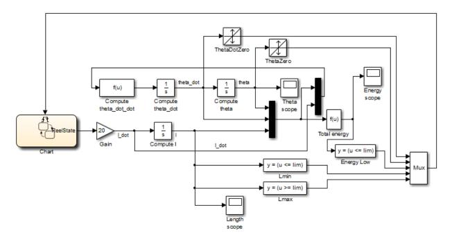
The chart contains two superstates: Active and Inactive. The Active state uses input events to guard transitions between different substates.
