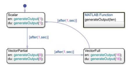
Use this Stateflow chart to generate an output signal with a variable size. In this chart, each state calls a MATLAB function that assigns to the chart output a different-size signal (within the bounds). During simulation, transitions between states change the size of the signal. You can use this variable-size signal to test other blocks and subsystems in your model.
