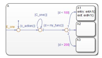
Initially, the chart is asleep. State A.A1 is active. The condition [C\_one()] is initially true. Event E\_one occurs and awakens the chart, which processes the event from the root down through the hierarchy:
