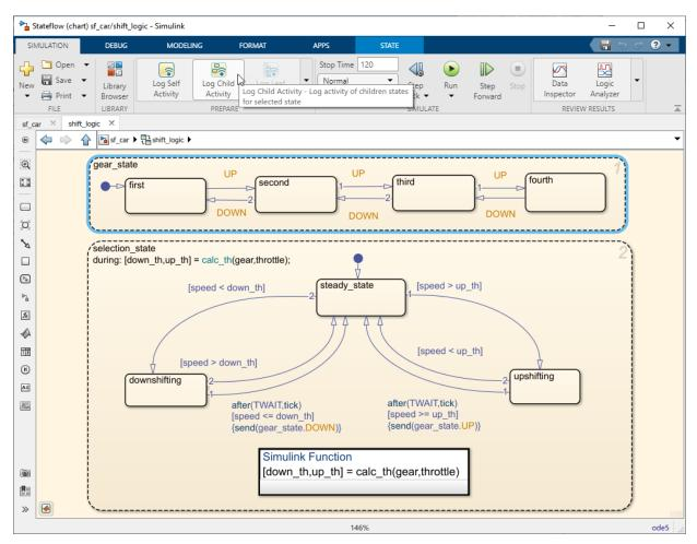
After running one or more simulations with signals marked for logging, click **Simulation**
