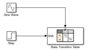
In the model, there is an event input and a data input. A Sine Wave block generates a repeating input event that corresponds with the Stateflow event SWITCH. The Step block generates a repeating pattern of 1 and 0 that corresponds with the Stateflow data object Shift. Ideally, the SWITCH event occurs at a frequency that allows at least one cycle through First, Second, and Third.
