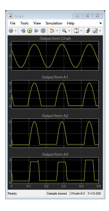
During each time step, the Ladder Logic Scheduler chart executes the subsystems depending on the values of the input signals u1 and u2:
