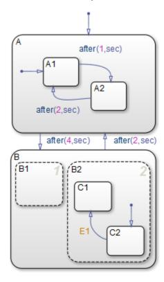
During simulation, a scope connected to the active state output data shows the enumerated values for the leaf states A1, A2, and B.
