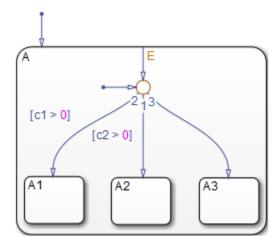
An event occurs and awakens the chart. The default transition to the connective junction is valid. The destination of the transitions is determined by [c1 > 0] and [c2 > 0].
