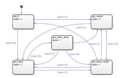
Before considering the value of coin, the Moore chart must compute the value of soda according to the active state. As a result, there is a delay in releasing soda, even if the machine receives enough money to cover the cost.
