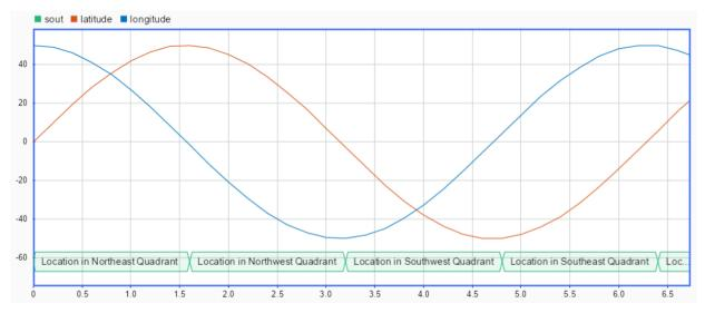
To access the logged data in the MATLAB workspace, call the signal logging object logsout. Stateflow exports the string data sout as a MATLAB string scalar. For example, at the command prompt, enter:
