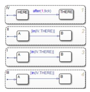
With this modification, the transitions from A to B occur in the same order as activation of the parallel states. For more information about the in operator, see "Check State Activity by Using the in Operator" on page 12-78.
