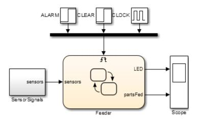
The chart now has only one input port on the left and an event triggered input on the top. For more information on how to create a Stateflow chart activated by events, see "Activate a Stateflow Chart by Sending Input Events" on page 10-9
