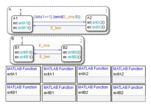
Initially, the chart is asleep. Parallel substates A.A1 and B.B1 are active, which implies that parallel (AND) superstates A and B are also active. The condition [datal==1] is true. The event E\_one belongs to the chart and is visible to both A and B.
