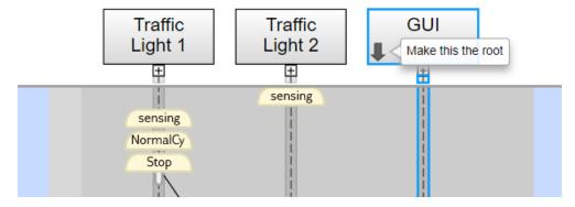
The Sequence Viewer window displays the current root lifeline path and shows its child lifelines. Any external events and messages are displayed as entering or exiting through vertical slots in the diagram gutter. When you point to a slot in the diagram gutter, a tooltip displays the name of the sending or receiving block.
