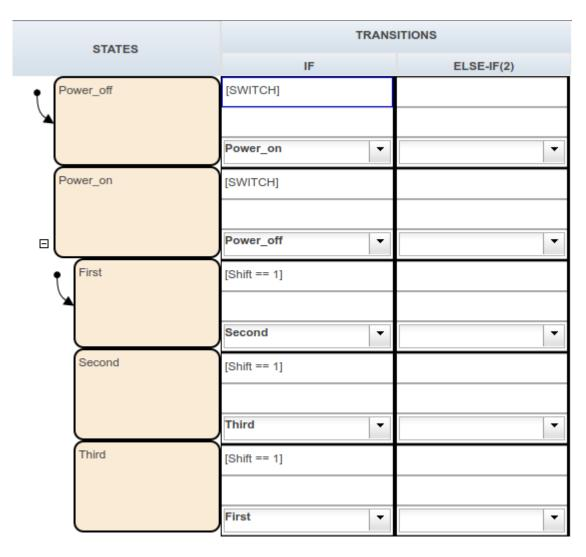
The table has two states at the highest level in the hierarchy, Power\_off and Power\_on. By default, Power\_off is active. The event SWITCH toggles the system between the Power\_off and Power\_on states. Power\_on has three substates: First, Second, and Third. By default, when Power\_on becomes active, First also becomes active. When Shift equals 1, the system transitions from First to
