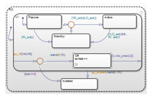
Another consequence if LO fails and moves out of Active is a transition that occurs in the right outer actuator (RO). The RO state transitions inside the L1 superstate from Active to Standby. This satisfies the requirement of the outer actuators and inner actuators to work in symmetry.
