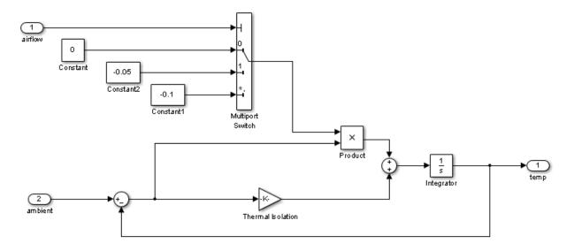
In this model, the internal temperature of the plant attempts to rise to achieve steady state with the ambient air temperature, set at a constant 160 degrees (as shown in "How the Stateflow Chart Works with the Simulink Model" on page 1-8). The rate at which the internal temperature rises depends in part on the degree of thermal isolation in the plant and the amount of cooling activity.
