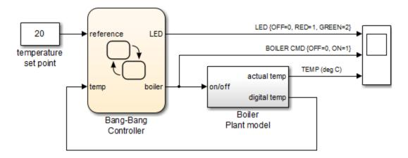
This model simulates for 1400 seconds, but the output that interests you occurs sometime between t = 400 and 600. You can simulate the model, save the operating point at time t = 400, and then load that operating point for simulation between t = 400 and 600.
