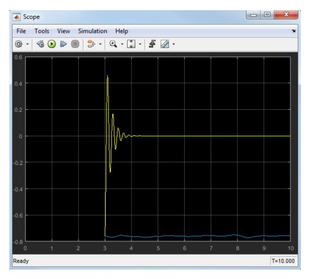
If you modify the operating point of your chart to test the response of the right elevator to actuator failures, you get similar results.
