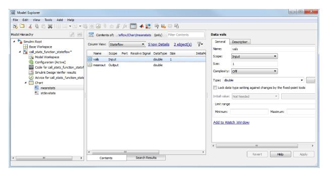
The function meanstats is highlighted in the **Model Hierarchy** pane. The **Contents** pane displays the input argument vals and output argument meanout. Both are scalars of type double by default.
