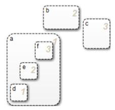
Because of explicit ordering, the priority of each state and substate matches the order of creation in the chart. The chart reprioritizes the parallel states and substates when you perform these actions:
