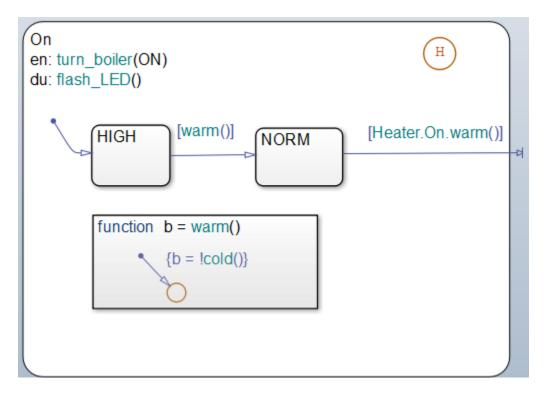
In this example, supertransition [Heater.On.warm()] goes from NORM in the On subchart to the Off state in the parent chart. Both segments of the supertransition have the same label.
