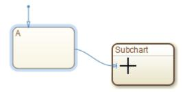
If you are not happy with the initial position of the slit, you can continue to drag the slit around the inside edge of the subchart to the desired location.
