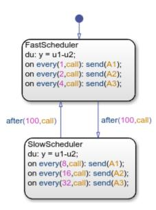
When the FastScheduler state is active, the chart schedules function calls to different Simulink subsystems at a fraction of the base rate at which the input event call wakes up the chart.
